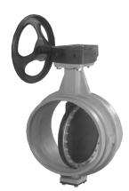
The Series W709 AGS (Advanced Groove System) grooved end butterfly valve offers an easily installed choice to cumbersome, multi-bolt wafer, lug-type or flanged valves. The valves has excellent flow characteristics with low torque operation. The resilient EPDM seat is rated for water services up to +230°F/+110°C. For services with oil content, the valve is available with Grade "T" nitrile seat, rated for petroleum, air with oil vapors, vegetable and mineral oils up to +180°F/+82°C.
