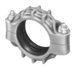
Style 77A aluminum couplings are designed with cross-ribbed construction. Providing a flexible connection, Style 77A is cast of an aluminum alloy prepared for strength and durability with minimum weight and is available in 1 - 8" (33,7 - 219,1 mm) and 12" (323,9 mm) sizes.
