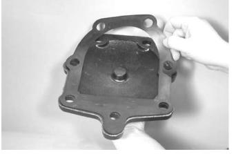
2. Align the holes of the cover plate gasket with the holes in the cover plate.
