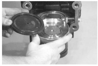
3. Remove the old solid seal from the clapper. Discard the solid seal.
