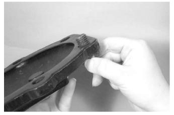
3. Insert one cover bolt through the cover plate and cover gasket to ease alignment.
