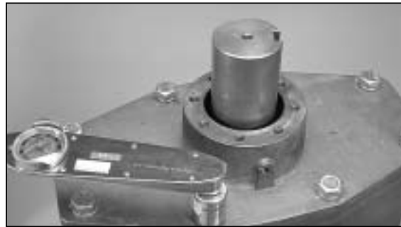
9. Install bonnet bolts (Item 19). Torque to 160 ft. lbs. (217.0 N•m) for 14 & 16" (350 & 400 mm) valves and 250 ft. lbs. (339.0 N•m) for 18" (450 mm) valve. Tighten in alternating criss-cross pattern.
