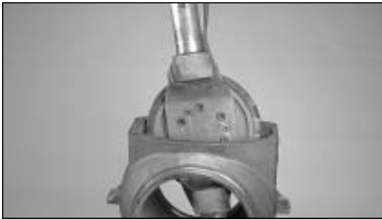
4. Place assembled plug and shaft into body. Rotate to ensure that the plug properly seats. Proper plug and shaft engagement is most easily accomplished with the plug and shaft in the open position.
