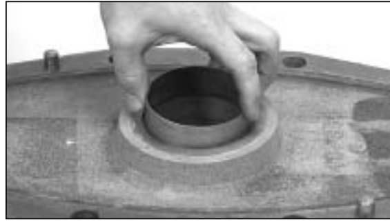
6. Install journal bearings (Item 9) into bonnet (Item 3). Apply silicone grease to the journal area
