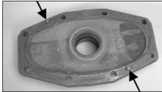
7. Note orientation of dowel pins (Item 14). Proper orientation of the bonnet with the dowel pins is necessary to permit bonnet reassembly.
