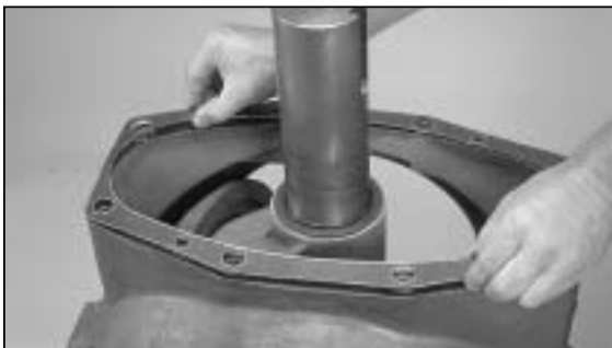
5. Place gasket (Item 8) on the top of the valve body (Item 1).
