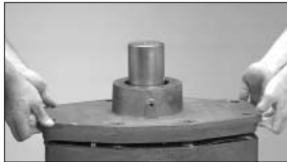
8. Install bonnet on top of body, making sure that the bonnet is correctly oriented and engaged on the dowel pins.
