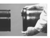
**3. INSTALL GASKET:** Place the large (NPS side) opening over the larger pipe end (NPS side). Be sure that the gasket lips do not overhang the pipe end.
