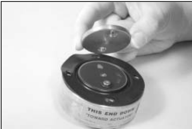
7. Remove the diaphragm retaining plate.
