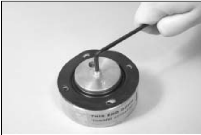
6. Using a \frac{9}{16} " hex wrench, remove the cap screw that retains the diaphragm assembly.
