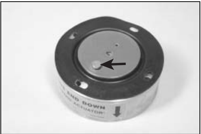
14. Install the NEW restrictor into the largest hole of the shield/diaphragm.
