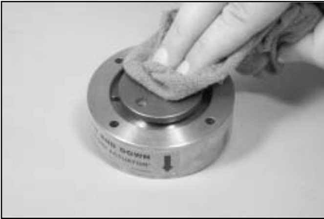
11a. Remove any debris or residue from the sealing areas of the lower housing with a non-abrasive cleaner.
