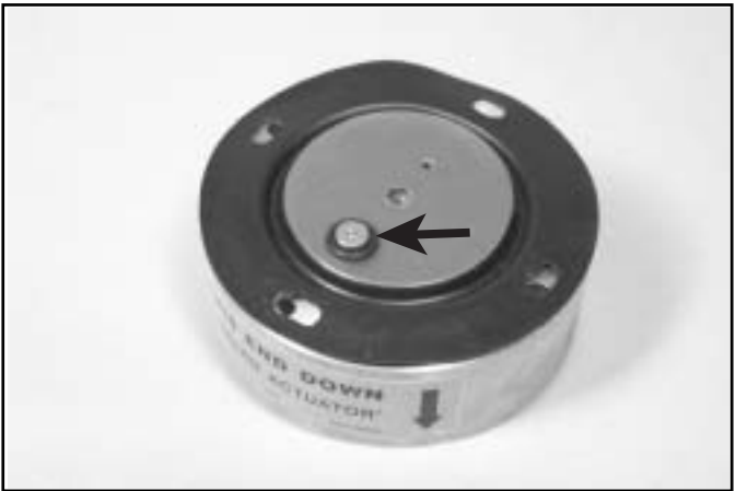
15. Install the NEW o-ring around the restrictor.
