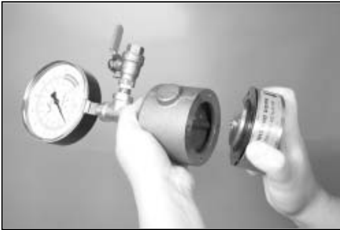
5. Separate the lower housing from the upper housing.
