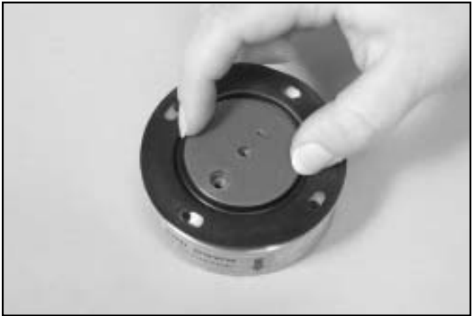
13. Install the NEW shield. Make sure the three holes in the shield align properly with the three holes in the diaphragm, as shown above.
