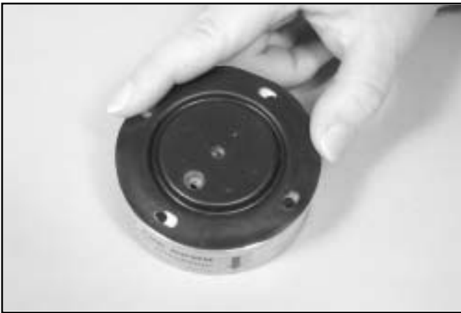
12. Install the NEW diaphragm onto the lower housing. Make sure the raised portion of the diaphragm is installed toward the lower housing. Make sure the largest hole in the center portion of the diaphragm aligns with the hole where the restrictor is normally installed, as shown above.
