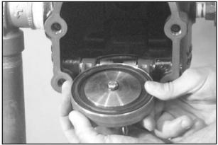
**5.** Rotate the clapper out of the valve body. Inspect the clapper seal and seal-retaining ring. Wipe away any contaminants, dirt, and mineral deposits. Clean any holes in the valve body seat ring that are plugged. **DO NOT USE SOLVENTS OR ABRASIVES.**
