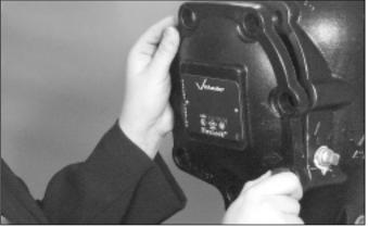
**2.** Align the cover plate and the cover plate gasket to the valve. Ensure that the spring arms are now rotated to their installed position. Insert the bolts by hand.
