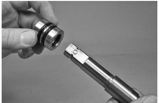
12. Insert the stem into the seal cartridge.
