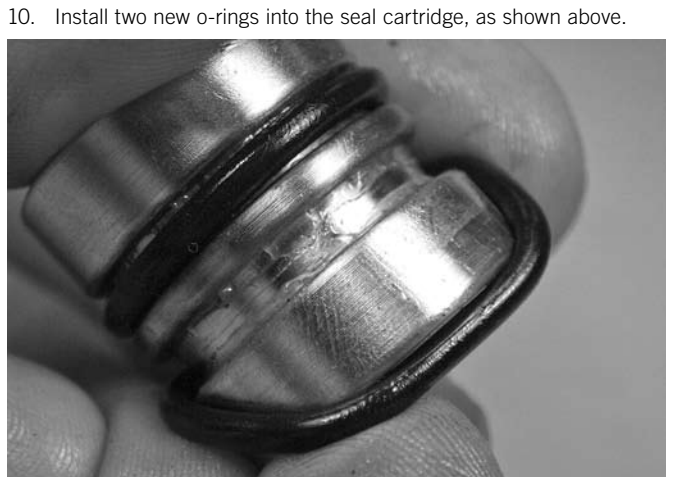
11. Install two new o-rings onto the seal cartridge, as shown above.
