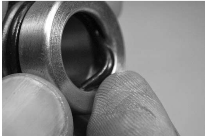
10. Install two new o-rings into the seal cartridge, as shown above.
