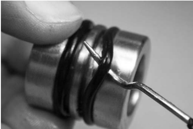
10. Install two new o-rings into the seal cartridge, as shown above.
