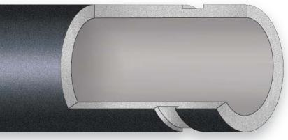
Cut groove shown on Schedule 80 carbon pipe. The groove created removes less metal than threading.
