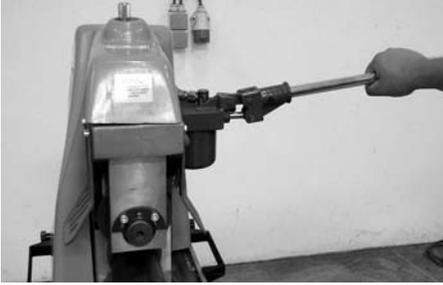
**5** Turn the groove diameter stop clockwise as far as possible. This is the zero-point.
