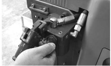
Hand pump valve closes automatically upon release.
