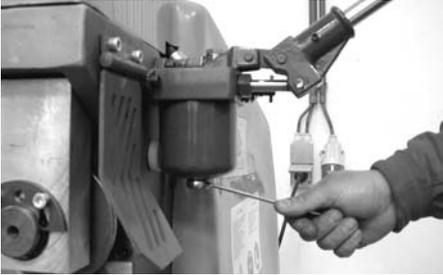
**2** Check the hydraulic fluid level and add oil as required.
