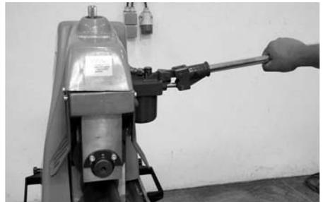
**4** Reconnect the hose to the hydraulic cylinder and tighten nut.
