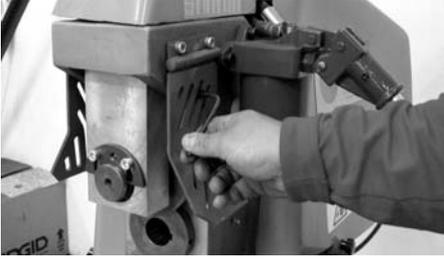
**7** Remove the roll removal tool from the upper shaft.
