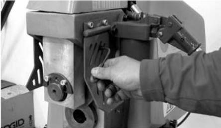
**2** With the 4 mm Allen wrench, loosen the cup point set screw in the upper roll.
