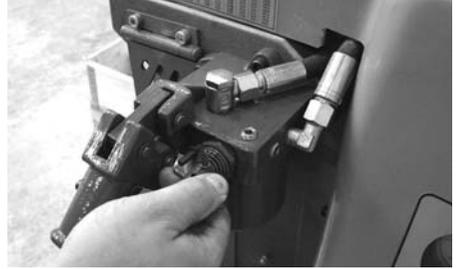
Hand pump valve closes automatically upon release.
