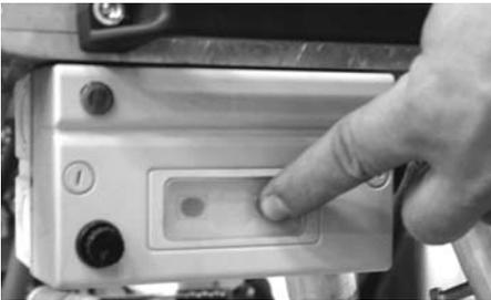
**3** Actuate safety foot switch by pressing foot on pedal to be certain tool is operational, power supply is available, and that lower roll is turning counterclockwise when viewed from the front. Remove foot from foot switch.
