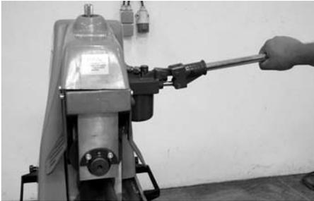
**7** If grooving a short pipe (see "Groovable Pipe Lengths"), remove hands from pipe.
