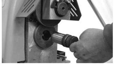
**3** With the 4 mm Allen wrench, tighten the cup point set screw in the lower roll.
