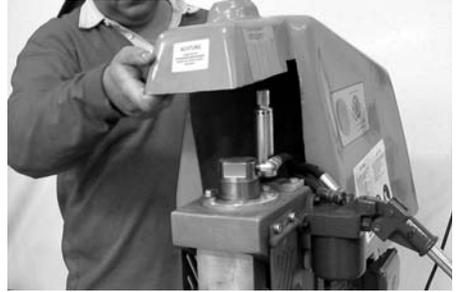
**2** Loosen the nut that connects the hose to the hydraulic cylinder. Remove the hose.
