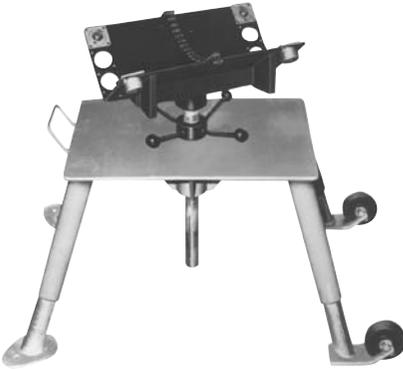
Victaulic Model VAPS 112 (art. code: R000112PS0), a portable, adjustable, roller type, four-leg pipe stand for use with Victaulic roll grooving tools, is available from Victaulic Europe. Ball transfer rollers, adjustable for pipe from 26,9 - 323,9 mm, will accommodate linear and rotational movement. Turnstile design permits easy swivel for grooving both pipe ends. Contact Victaulic Europe for details.
