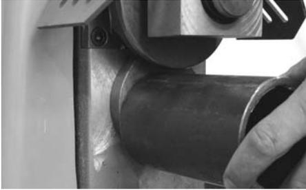
**6** Pump the handle several times to bring the upper roll into light but firm contact with the pipe.
