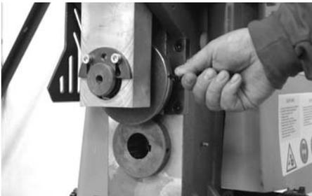
**3** With the 6 mm Allen wrench, loosen the 2 adjustment screws and slide the distance plate up, away from the upper shaft.
