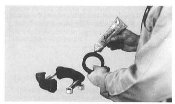
MAKE SURE BALL VALVE IS FULLY OPEN. Remove gasket from the 2½" HP-70 and lubricate with Vic-Lube as shown.
