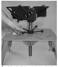
**5.** Adjust the V-shaped pipe trough to the approximate height necessary for grooving using the height adjusting nut.
