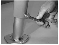
**4.** Adjust the leg height using the height adjusting nut.
