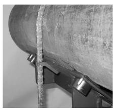
**7.** Connect the safety chain loosely over the top of the pipe.
