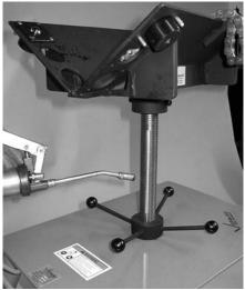
**2** On a monthly basis, raise the pipe stand to its maximum height and grease the threaded height adjusting rod by applying #2EP Lithium base grease to the exposed threads.
