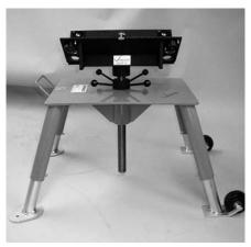
**2a.** Work in the grease by lowering the stand to its minimum height.
