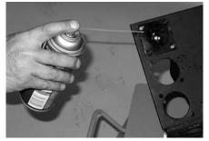
**1.** Regular lubrication is required for the VAPS112 pipe stand. On a weekly basis, apply a few drops of light oil to the ball transfer units. Work the oil in by rotating the units.
