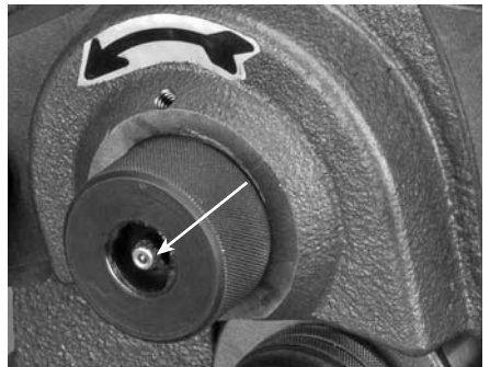
5. After every 8 hours of operation, apply grease to the grease fitting of the upper roll shaft.
