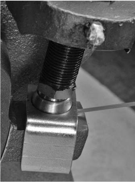
2. Apply grease underneath the toggle pad.
