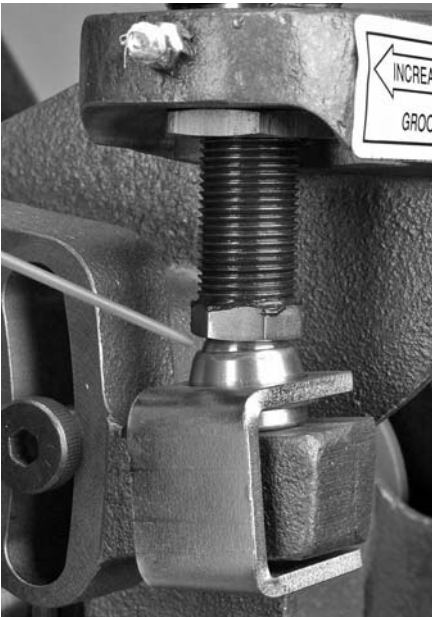
3. Apply grease to the ball-and-socket joint of the toggle pad.
