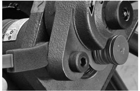
4. Apply grease to the locations where the roll arm slides against the tool body.
