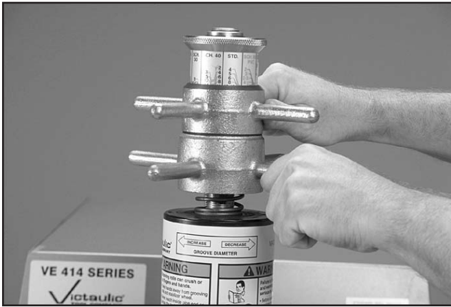
12. Set the depth stop on the tool to obtain approximately a 1/4-inch (5-mm) gap between the depth stop and the cylinder.
