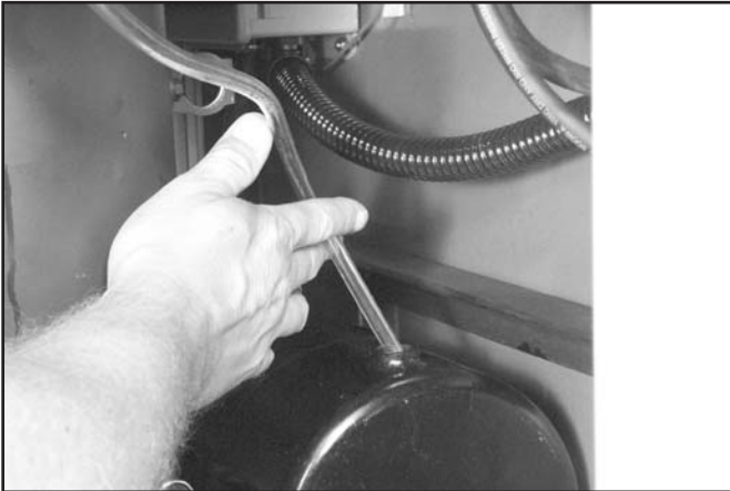
5. Insert the end of the bleeder tube (clear hose) into the tank so that the end is submerged in the hydraulic fluid.
